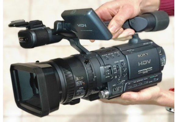
The Sony FX1 could be used to shoot HD as well as SD to Mini DV tape, an eye-opener in 2004
