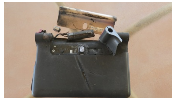
The damage results of a Lenovo Tablet after the explosion
