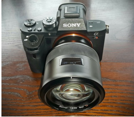
The 85/1.8 Zeiss Batis without its lens hood. The OLED panel on the lens displays the focused distance and depth of field. The display can be switched between Imperial and metric
