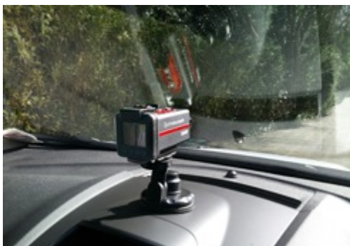
Camera fixed to the top of the car's instrument panel. Note the high level of reflections from the screen when shooting into the light
