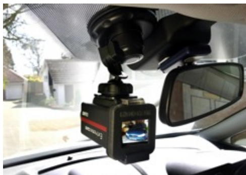
Camera fixed to the top of windscreen. pPreferred position as long as the wipers clear this portion of the screen. Footage recorded upside-down.
