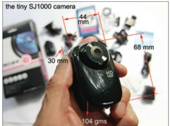
There's a comprehensive menu that allows you to set the camera up in various guises. You can loop-record so that when the class 4 Micro SDHC card is full (a 16gb card will hold just over 2 hours of full HD) the camera will then over-write the earliest segment and continue
