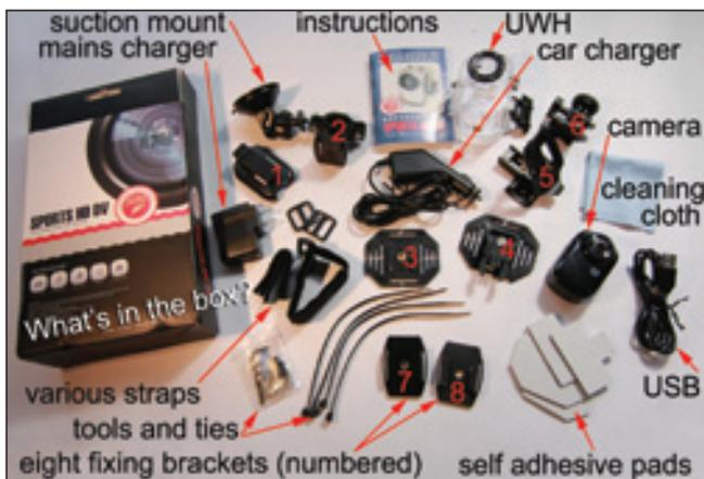
Take a look at my photo 'What's in the Box?' I opened it and out fell about 21 components, consisting of a vast array of brackets, stands, clamps, straps, cables, ties, the camera itself, an under-water housing (UWH), instructions, a car and mains charger. The camera itself is about 2¾" high and somewhat resembles a smooth rounded pebble, with a very wide-angle lens sitting in a small protrusion. I chose a black one, but prettier versions are available in various colours. It has
